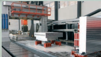
In-ground gantry machine machining of aluminium
