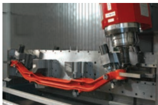
Machining of truck axles on matec-40 HV
