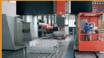
In-ground gantry machine with traveling operator platform
