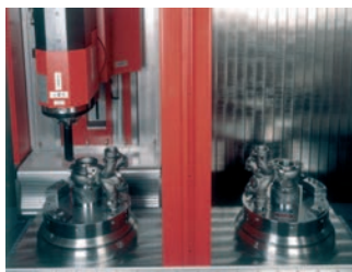
matec-30 HVT: 2 working areas - mounted rotary tables with direct drive
