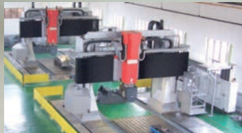
In-ground gantry machines allow the machining of very voluminous parts and high-speed milling
