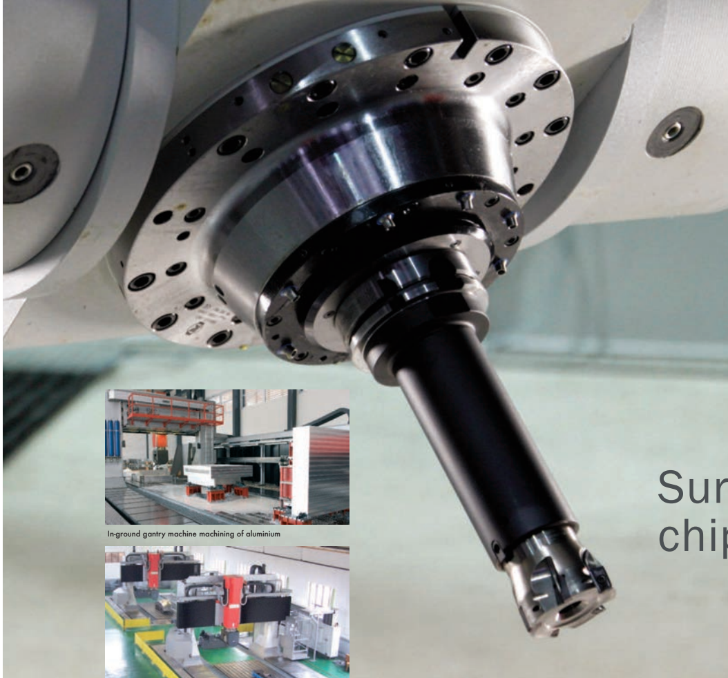
In-ground gantry machines allow the machining of very voluminous parts and high-speed milling
